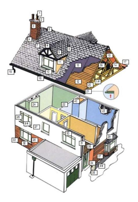
3 Chimney head Flashing 4 Ridge ventilation 5 Ridge board Slates/tiles 8 Valley guttering 9 Dormer projection Dormer flashing 10 Dormer cheeks 11 12 Sarking Roof felt 13 Trusses 14 15 Collar 16 Insulation
