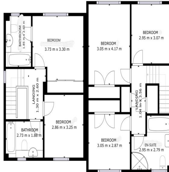
FIGURE 2 GROSS INTERNAL AREA FLOOR 1: 118.07 M 2 ; FLOOR 2: 16.41 M 2 TOTAL: 134.48 M 2 NOTE: ALL DIMENSIONS ARE APPROXIMATIONS. ACTUAL MAY VARY.
